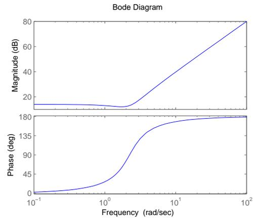
The bode plot of  $s^2 - 2s + 5$  is below; this is a non-minimum-phase system, with unstable zeros.
