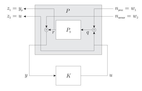
The plant P is given by  $\begin{bmatrix} z_1 \\ z_2 \\ y \end{bmatrix} = \begin{bmatrix} P_0 & 0 & P_0 \\ 0 & 0 & 1 \\ P_0 & 1 & P_0 \end{bmatrix} \begin{bmatrix} w_1 \\ w_2 \\ u \end{bmatrix}$ Suppose  $P_0$  is  $\dot{x} = Ax + Bq$ r = Cx + Dq
