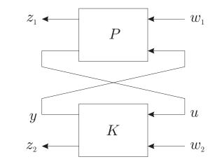
$S(P, K) = \begin{bmatrix} \underline{S}(P, K_{11}) & P_{12}(I - K_{11}P_{22})^{-1}K_{12} \\ K_{21}(I - P_{22}K_{11})^{-1}P_{21} & \overline{S}(K, P_{22}) \end{bmatrix}$
