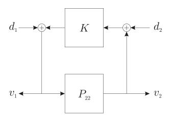
Inject actuator and sensor noise  $d_1$  and  $d_2$ . Then
