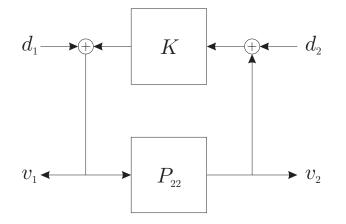
Suppose the realizations for  $P_{22}$  and K are stabilizable and detectable. Then the above feedback loop is internally stable if and only if
